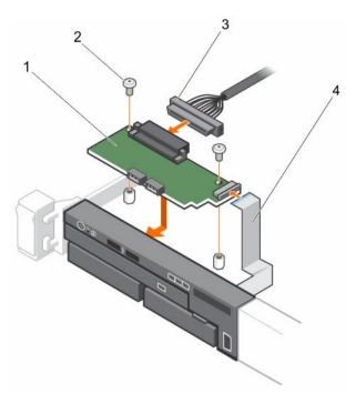
Figure 98. Installing the control panel module—eight hard-drive chassis
