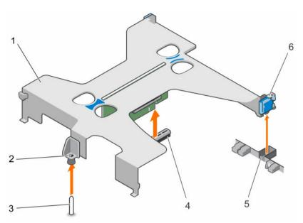
Figure 50. Removing and installing the expansion card riser
