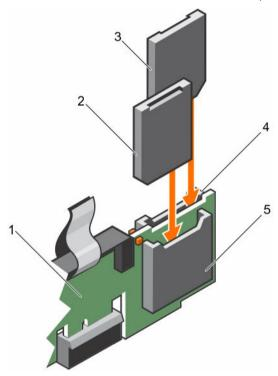
Figure 59. Installing an internal SD card
