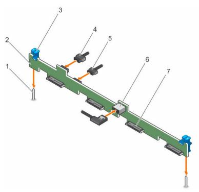
Figure 84. Installing the four 3.5 inch hard drive SAS/SATA backplane
