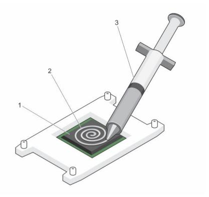
Figure 68. Applying thermal grease on the top of the processor
