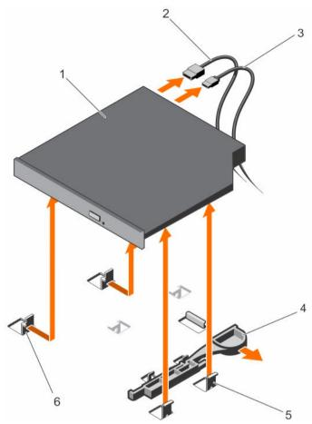
Figure 44. Removing the standard optical drive
