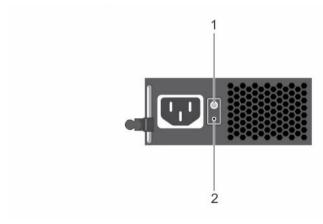
Figure 15. Non-redundant AC PSU status indicator and self-diagnostic button
