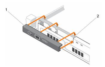
Figure 90. Installing the control panel—four 3.5 inch hard-drives chassis
