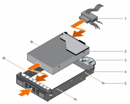
Figure 33. Installing a cabled hard drive carrier
