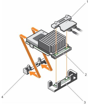
Figure 63. Installing the integrated storage controller card
