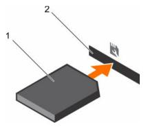
Figure 57. Installing an optional SD vFlash card
