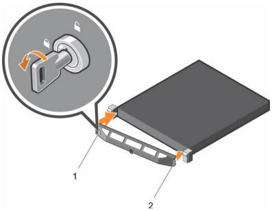
Figure 18. Installing the optional front bezel
