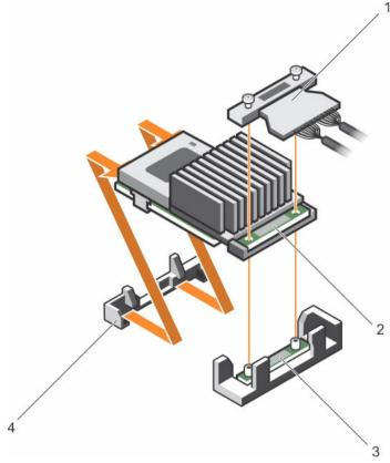
Figure 62. Removing the integrated storage controller card
