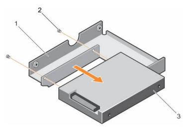
Figure 38. Removing a 2.5-inch hard drive from a 3.5-inch hard drive adapter
