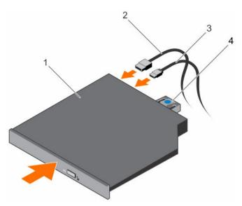
Figure 43. Installing the ultra slim optical drive
