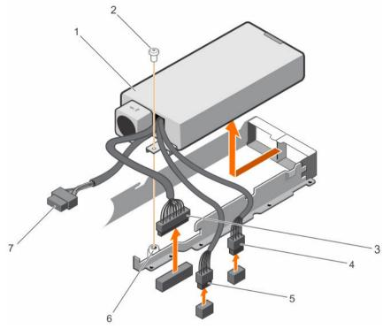
Figure 72. Removing a cabled PSU
