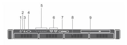
Figure 3. Front panel features of the 4 x 3.5 inch cabled hard drive system
