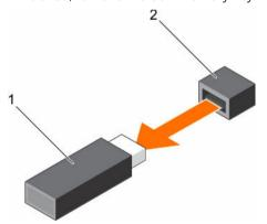
Figure 48. Removing the internal USB memory key
