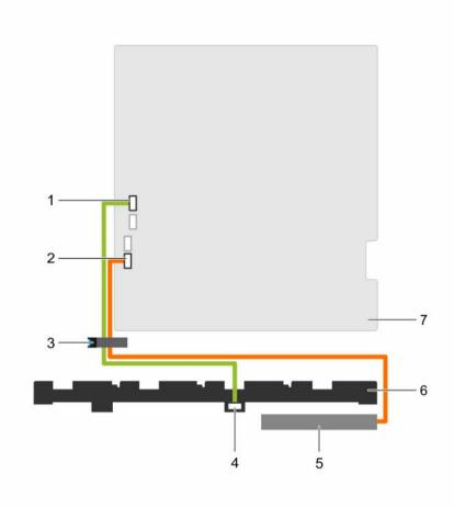
Figure 79. Cabling diagram—Four 3.5 inch or 2.5 inch hard drive SAS/SATA backplane
