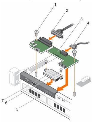
Figure 96. Installing the control panel module—four cabled hard-drive chassis
