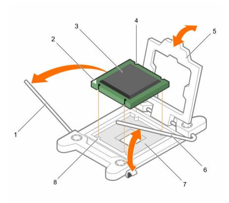
Figure 66. Removing a processor
