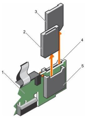
Figure 58. Removing an internal SD card
