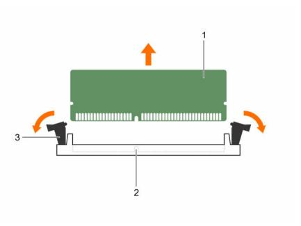
Figure 26. Removing the memory module
