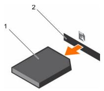
Figure 56. Removing the optional SD vFlash card
