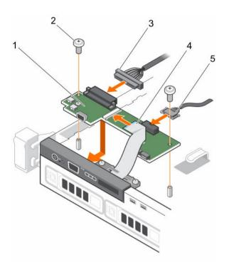
Figure 97. Installing the control panel module—four hard-drive chassis
