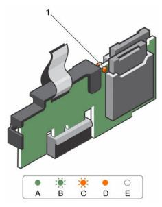
Figure 12. Internal dual SD module (IDSDM)
