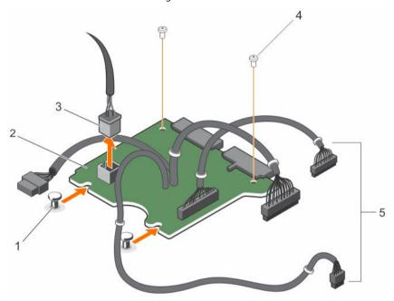
Figure 99. Removing the power interposer board
