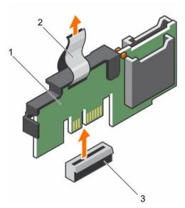
Figure 60. Removing the internal dual SD module (IDSDM)
