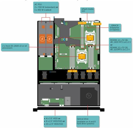
Figure 1. Supported configurations for the PowerEdge R430 system
