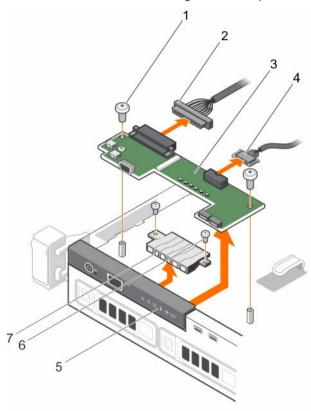
Figure 93. Removing the control panel module—four cabled hard-drive chassis
