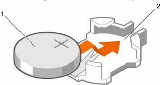
Figure 77. Installing the system battery
