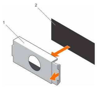
Figure 74. Removing the PSU blank
