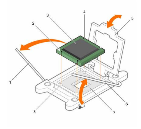
Figure 67. Installing a processor
