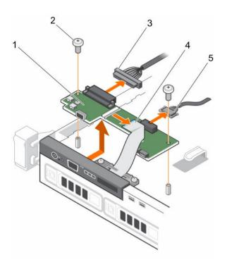
Figure 94. Removing the control panel module—four hard-drive chassis
