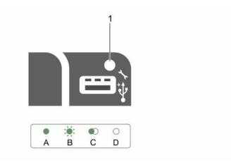
Figure 13. iDRAC Direct LED indicator
