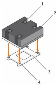
Figure 69. Installing the heat sink
