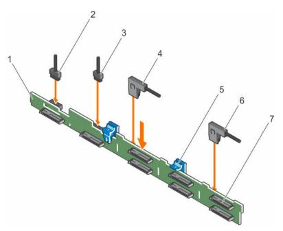
Figure 85. Installing the eight 2.5 inch SAS/SATA backplane
