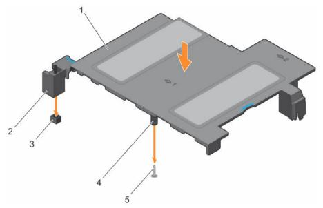
Figure 24. Installing the cooling shroud
