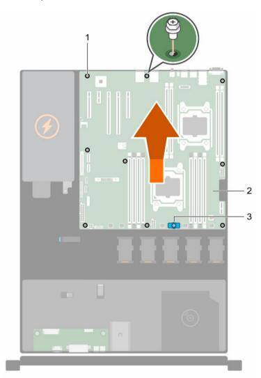
Figure 101. Removing the system board
