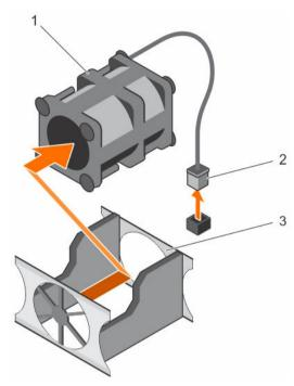
Figure 46. Removing a cooling fan
