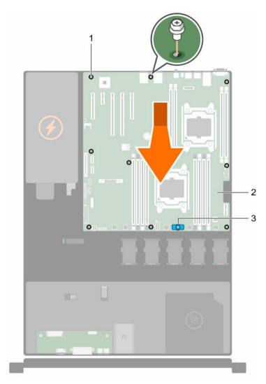
Figure 102. Installing the system board
