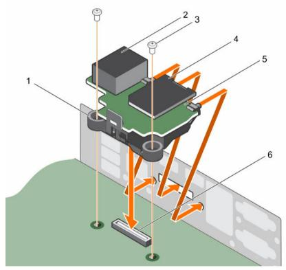
Figure 55. Installing the iDRAC port card
