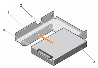
Figure 39. Installing a 2.5-inch hard drive into a 3.5-inch hard drive adapter
