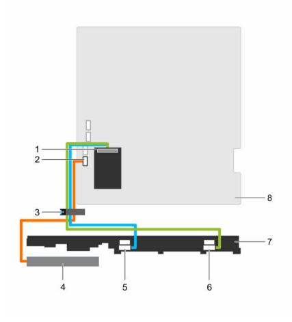
Figure 81. Cabling diagram—Eight 2.5 inch SAS/SATA backplane
