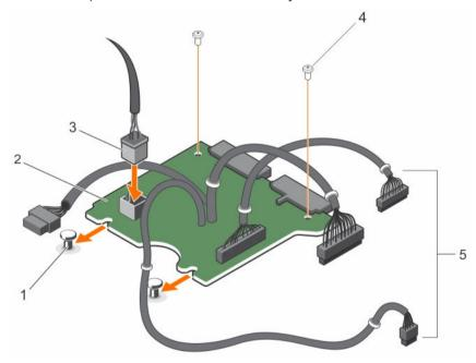
Figure 100. Installing the power interposer board
