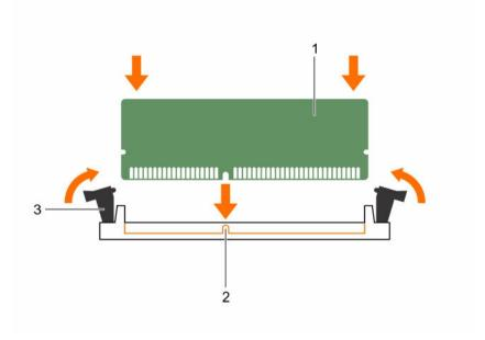
Figure 27. Installing the memory module
