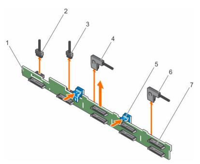
Figure 80. Removing the eight 2.5 inch SAS/SATA backplane
