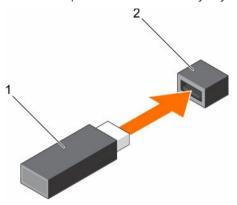
Figure 49. Installing the internal USB memory key
