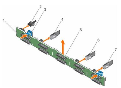
Figure 82. Removing the ten 2.5 inch SAS/SATA backplane
