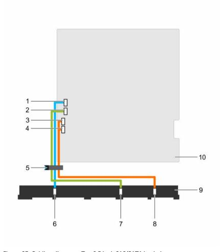
Figure 83. Cabling diagram—Ten 2.5 inch SAS/SATA backplane
