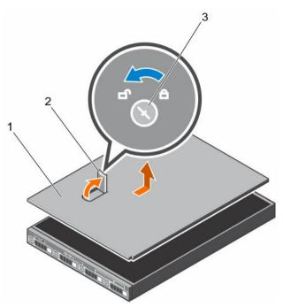
Figure 19. Removing the system cover
