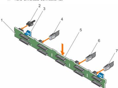
Figure 86. Installing the ten 2.5 inch SAS/SATA backplane
