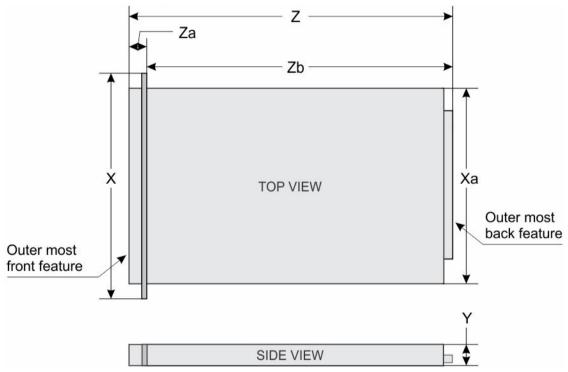
Figure 16. Chassis dimensions of the PowerEdge R430 system
