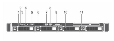
Figure 2. Front panel features of a 4 x 3.5-inch hard drive system
