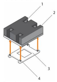
Figure 64. Removing a heat sink
