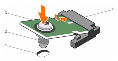
Figure 103. Installing the TPM
