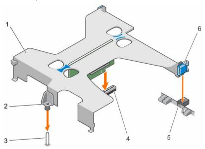
Figure 51. Installing the expansion card riser
