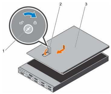
Figure 20. Installing the system cover
