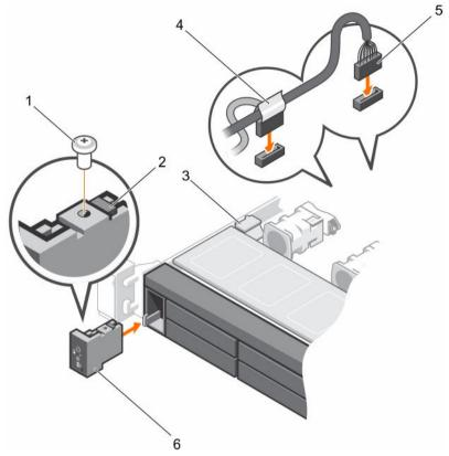
Figure 92. Installing the control panel—ten 2.5 inch hard-drives/SSDs chassis
