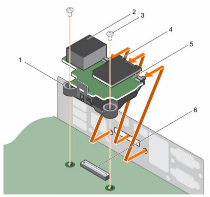
Figure 54. Removing the iDRAC port card
