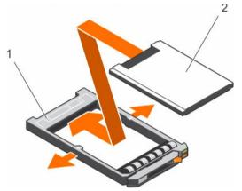
Figure 40. Installing a 1.8-inch hard drive into a hard drive carrier
