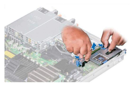
Figure 44. Removing the expansion riser 1B
