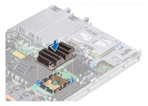
Figure 43. Installing a processor and heat sink module
