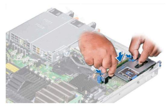
Figure 49. Installing the expansion riser 1B
