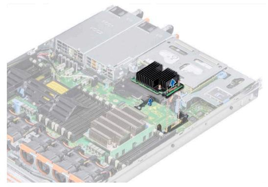
Figure 68. Removing the integrated storage controller card
