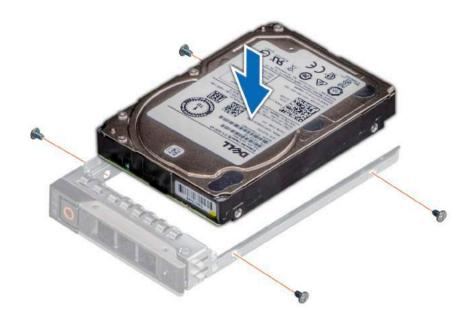
Figure 76. Installing a hard drive into the hard drive carrier
