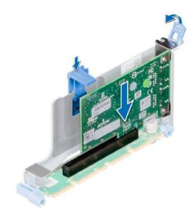
Figure 60. Installing an expansion card into the expansion riser 1B
