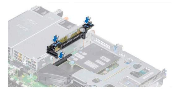
Figure 50. Installing the expansion riser 2A
