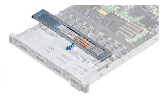
Figure 24. Installing the backplane cover
