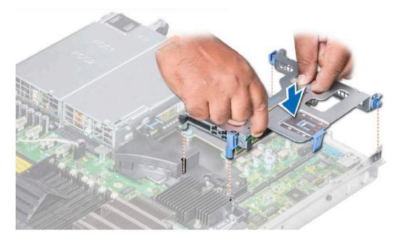
Figure 48. Installing the expansion riser 1A
