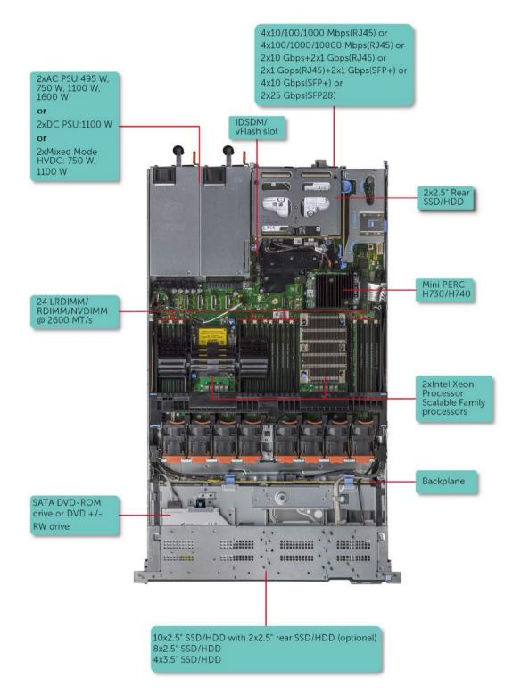
Figure 1. Supported configurations for PowerEdge R640
