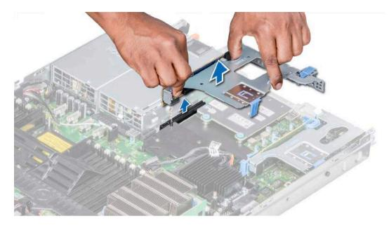
Figure 47. Removing the expansion riser 2B
