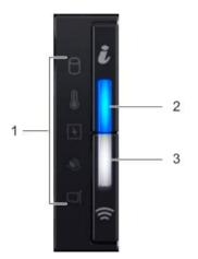
Figure 5. Left control panel with optional iDRAC Quick Sync 2.0 indicator
