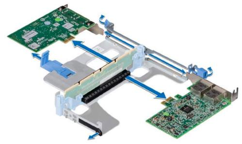
Figure 52. Removing an expansion card from riser 1A
