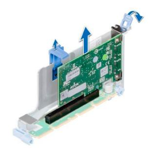
Figure 53. Removing an expansion card from riser 1B
