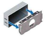
Figure 98. Removing a power supply unit blank
