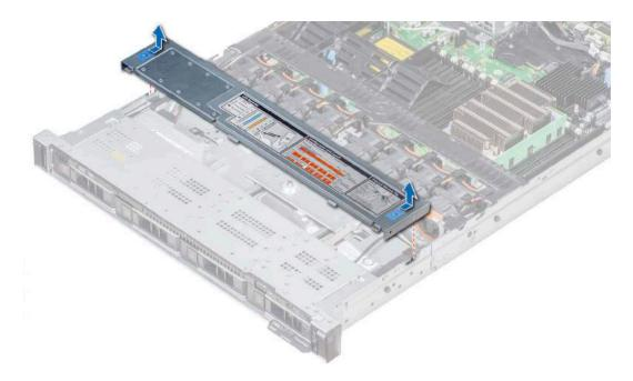
Figure 23. Removing the backplane cover
