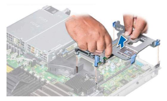
Figure 45. Removing the expansion riser 1A
