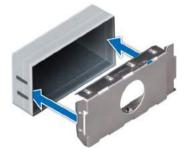
Figure 99. Installing a power supply unit blank
