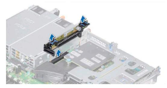
Figure 46. Removing the expansion riser 2A
