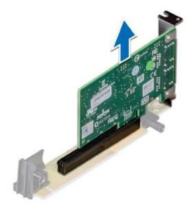
Figure 54. Removing an expansion card from riser 2A
