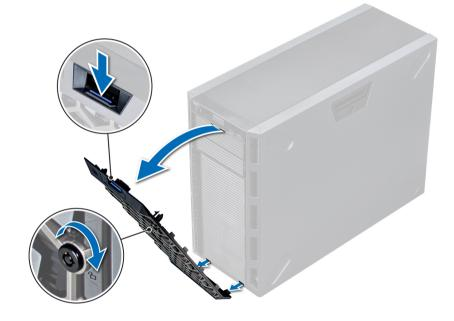
Figure 13. Removing the front bezel
