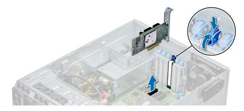
Figure 58. Removing an expansion card
