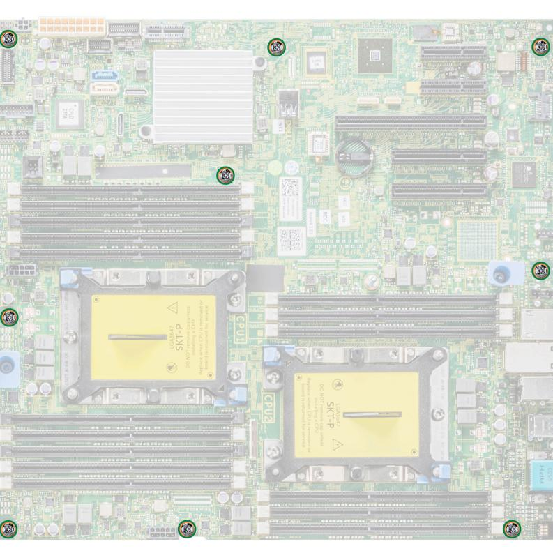
Figure 84. System board screws
