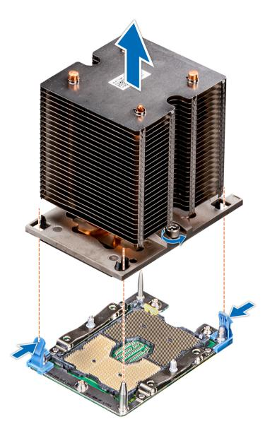
Figure 64. Removing the processor and heat sink module
