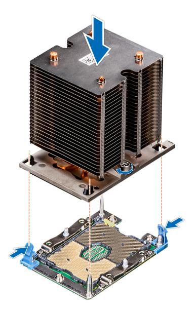
Figure 70. Installing a processor and heat sink module
