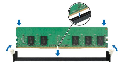
Figure 51. Installing a memory module
