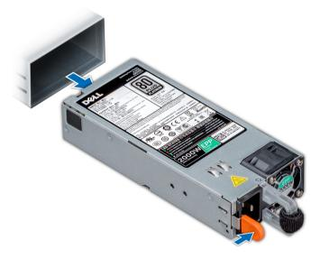
Figure 73. Removing a power supply unit
