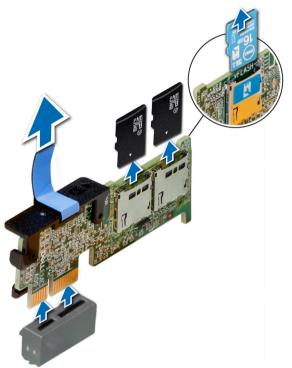
Figure 62. Removing the optional IDSDM/vFlash card
