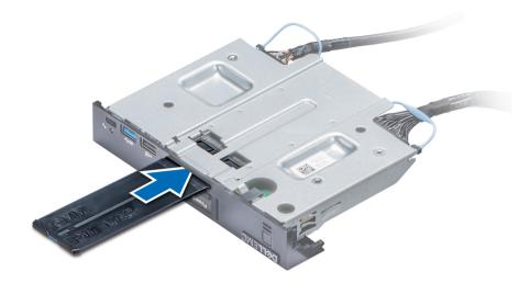
Figure 82. Installing the information tag
