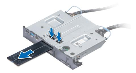
Figure 102. Removing the information tag
