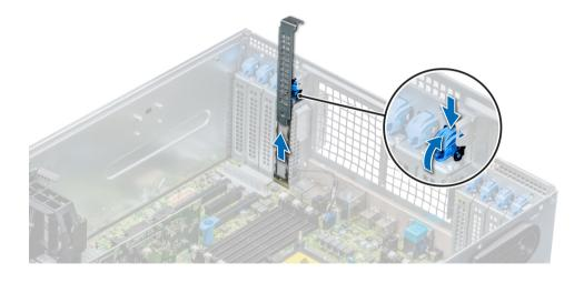
Figure 71. Removing the filler bracket
