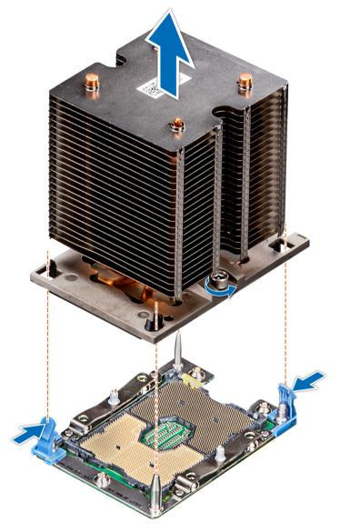
Figure 58. Removing the processor and heat sink module
