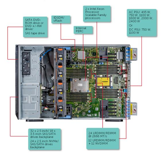
Figure 1. Supported configurations of the PowerEdge T640
