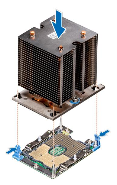
Figure 64. Installing a processor and heat sink module
