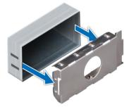
Figure 31. Removing a power supply unit blank
