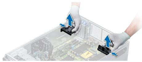
Figure 65. Removing the expansion card holder
