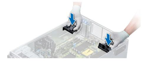
Figure 66. Installing the expansion card holder
