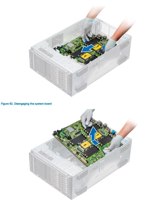
Figure 93. Removing the system board
