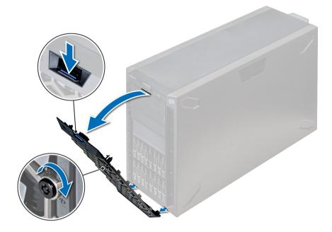
Figure 15. Removing the front bezel
