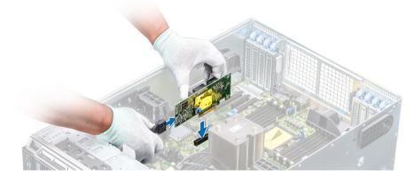
Figure 88. Installing the integrated storage controller card
