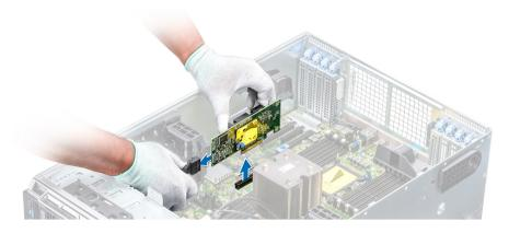
Figure 87. Removing the integrated storage controller card
