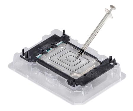
Figure 62. Applying thermal grease on top of the processor
