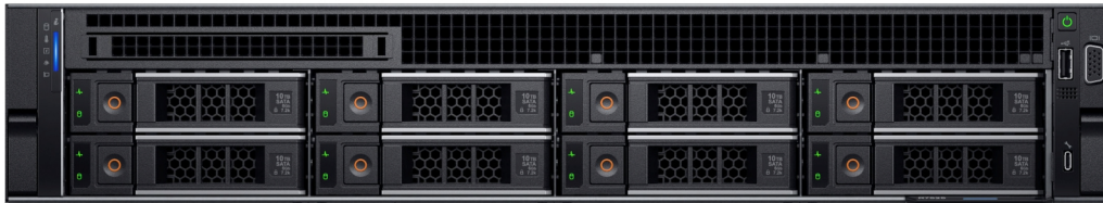
Figure 1. Front view of 8 x 3.5-inch drive system
