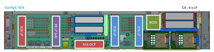
Figure 11. Rear view of the system
