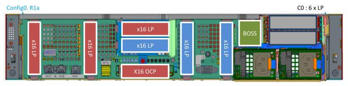
Figure 8. Rear view of the system with riser slot numbering
