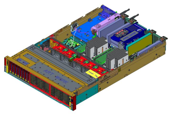
Figure 13. Inside the 8 x 2.5-inch system
