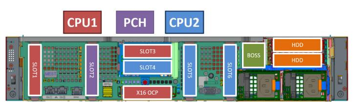
Figure 7. Rear view of the system
