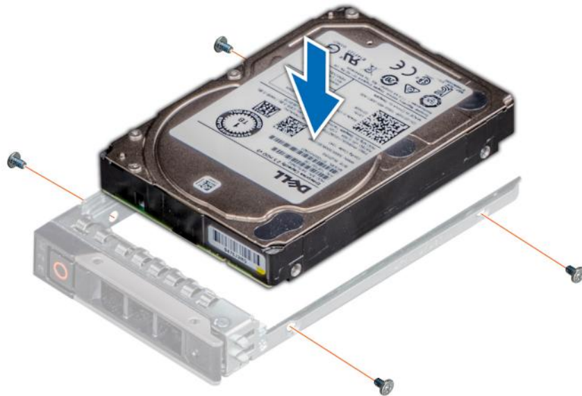
Figure 64. Installing a drive into the drive carrier
