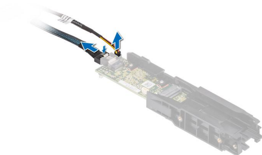
Figure 149. Removing the BOSS-N1 power and signal cable from the BOSS-N1 module
