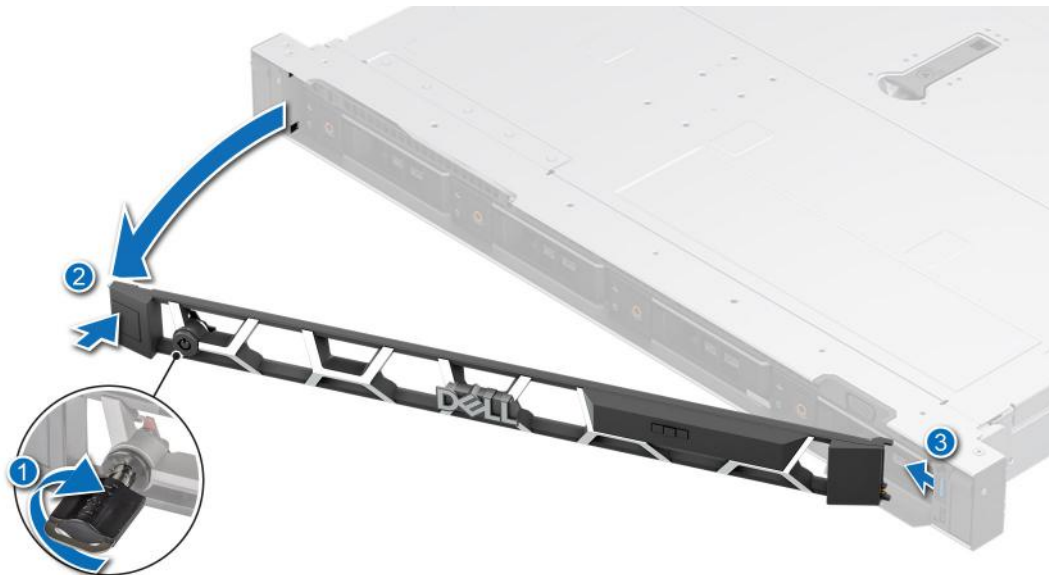
Figure 46. Installing the front bezel with the LCD panel
