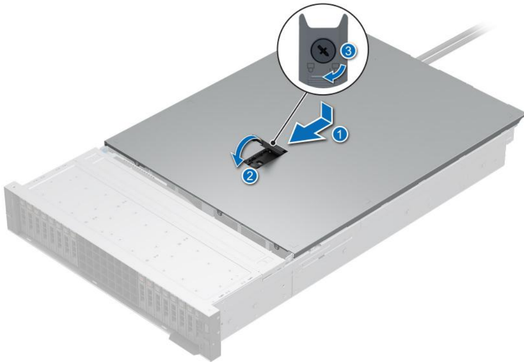
Figure 33. Installing the system cover
