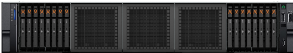
Figure 7. Front view of 16 x EDSFF E3.S
