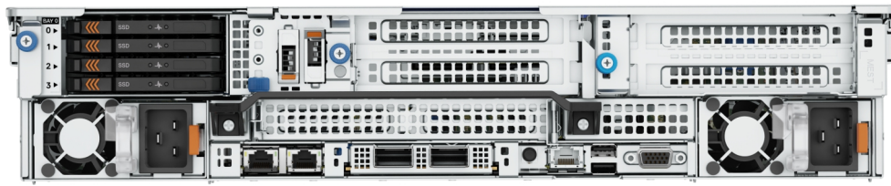
Figure 13. Rear view of the system with 4 x EDSFF E3.S rear drive module
